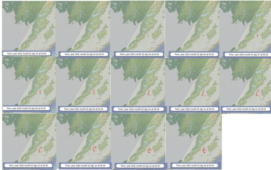
Figure 5. A particle tracking experiment run with ICHTHYOP 3.1 Stable version. The radius of the stain was 15 km.
